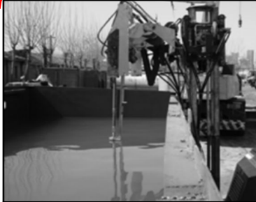
图5 淹没环境高压水射流破碎混凝土实验设备 Fig.5 Experiment Device of Removing Concrete
